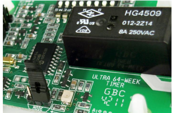
however if the door is open after the 3 minutes the relay will activate - if auto link is fitted relay drops out after 20 seconds and is then “waiting for next trigger”
